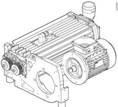
3. Install the pulley to the motor.
