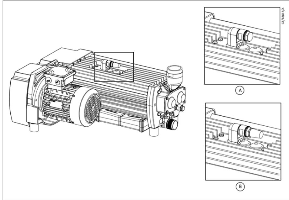
A. Gas ballast closed (blind plug installed)
