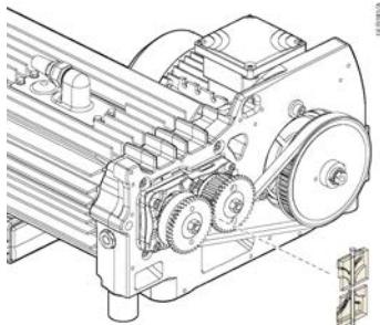
10. Assemble the fail safe gears bolts and tighten with 10 Nm .
