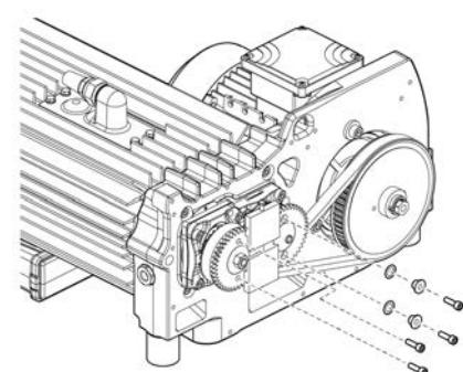
7. Remove the gear fixation tool.
