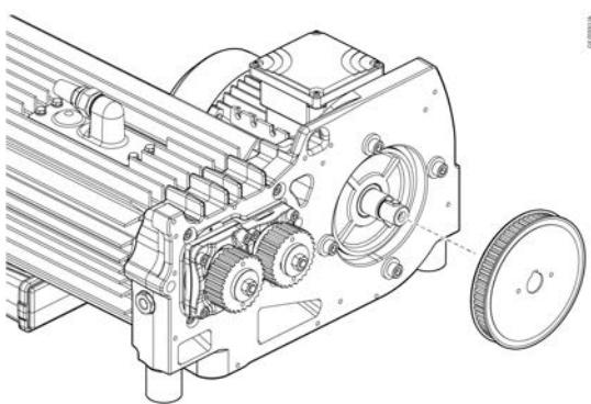
5. Tap the pulley with a mallet gently to push the pulley.
