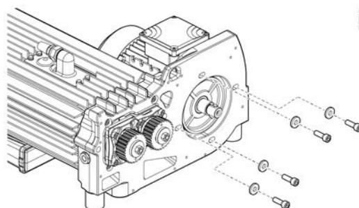
4. Make sure that the key (1) and keyway are aligned correctly.
