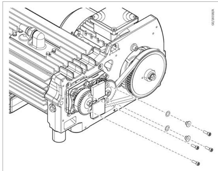
4. Remove the gear adjustment tool.
