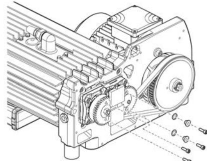
11. Fix the centre nut. Use a torque wrench to tighten the screw to 25 Nm.
