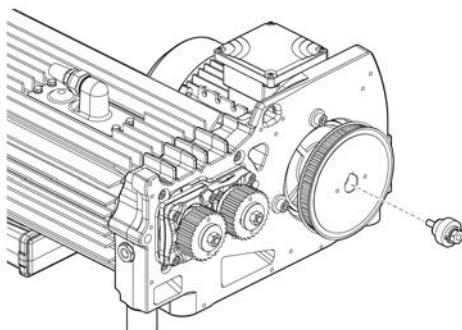
13. Install the gear puller into the middle of the pulley.
