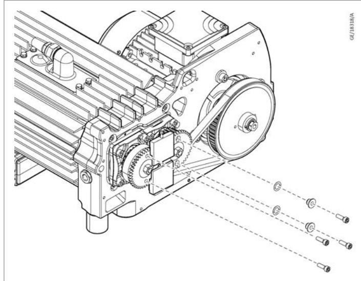
5. Remove the gear adjustment tool.
