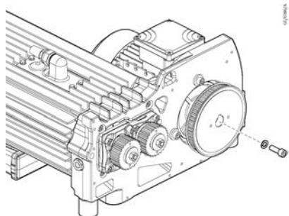
14. Remove the pulley with the gear puller tool and M8 hexagonal screw.
