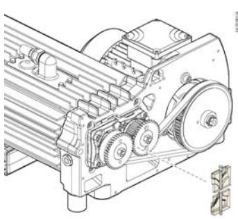
8. Remove the fail safe gears.
