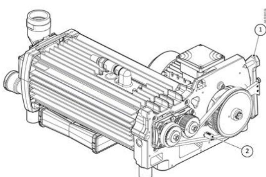
2. Install the 4 motor screws and hand tighten.
