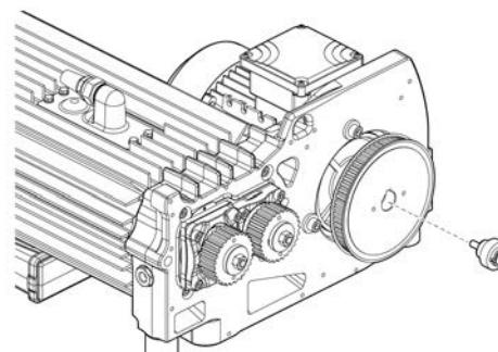
8. Assemble both fail-safe gears. Replace the plastic fail-safe gear if it is worn.
