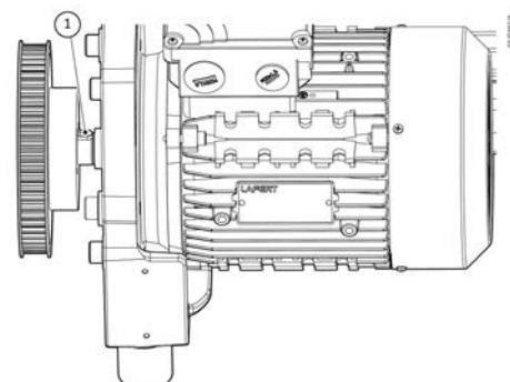
6. Insert the centre screw and hand tighten.
