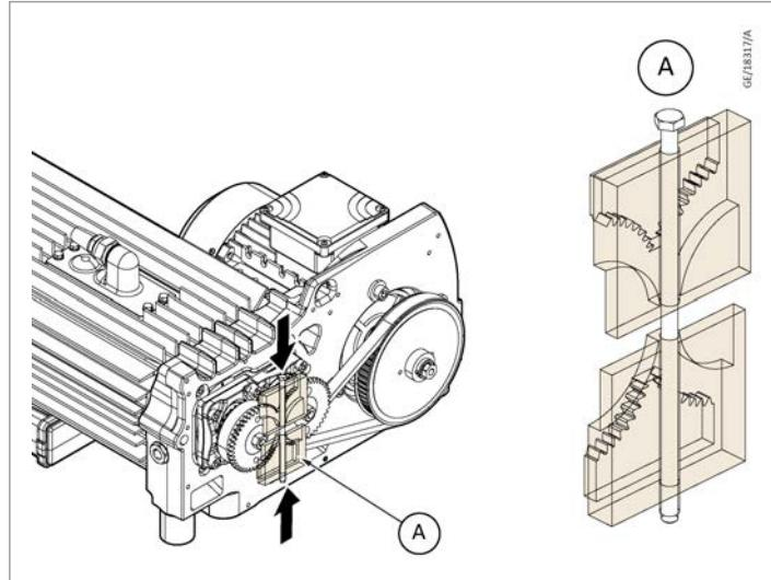
3. Loosen the 4 bolts fixing the gears with a 5 mm Allen key and remove the bolts.
