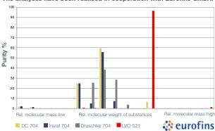
A low relative molecular mass and mixtures of various substances in the oil interfere with the performance of diffusion pumps. LVO 521 contains a very high-purity of a special silicone to help you to get the best performance from your pump.
