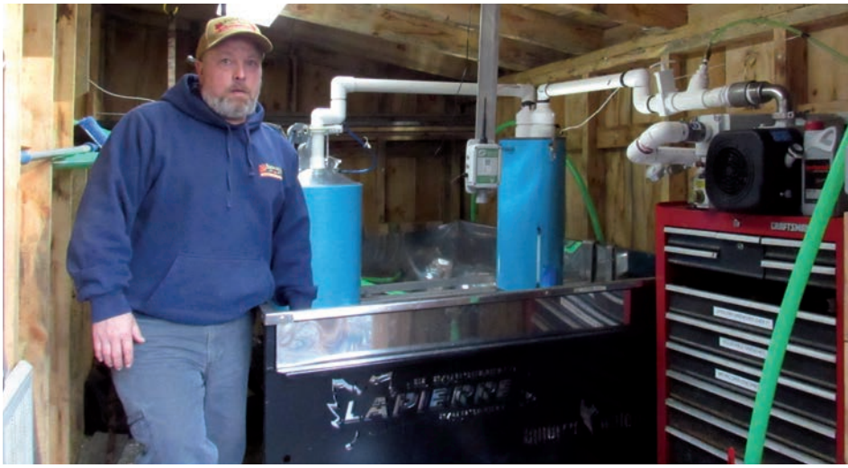
A view into the pump house shows a typical maple sap vacuum pump installation. Vacuum pump, moisture trap, sap vacuum extractor, that connects to the tubing in the woods. And the maple sap tank in which the extractor dumps maple sap.
